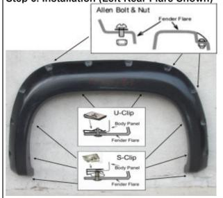
Use torx bit to tighten allen bolt & put firmly on every pocket of the fender flares. DO NOT OVER TIGHTEN! Hold the flare in position on the vehicle, use a grease pencil to mark eight hole locations. Apply 2 U-Clips over two top marks, align with holes in flare. Apply 6 S-Clips over six lower marks, align with holes in flare. Adjust the clips in position, use 2 flange screws and 6 truss maching screws to secure it as shown.
